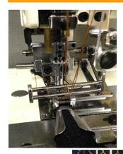
Design of the smocking can be easily changed from backside of the machine by changing the cam, changing thread variation
