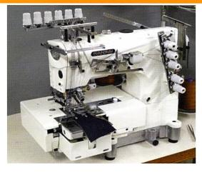
3 needle, flatbed, bottom cover-stitch, belt-loop making machine with front fabric knife and 2 spreader 6 thread smocking mechanism
